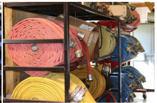
Synthetic fiber and plastic-lined fire hoses made from petro-chemicals are stronger, easier to maintain and more reliable than their older cotton fabric predecessors.
